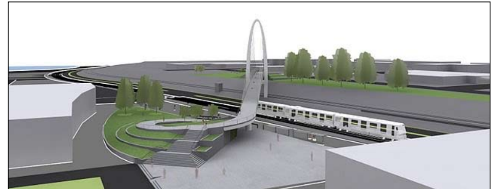
FIGURE 4.6: BICYCLE & PEDESTRIAN BRIDGE: CABLE-STAYED OPTION
