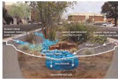
Depressed median for stormwater treatment (Bernalillo County [NM] Technical Standards App. A, 2022)
